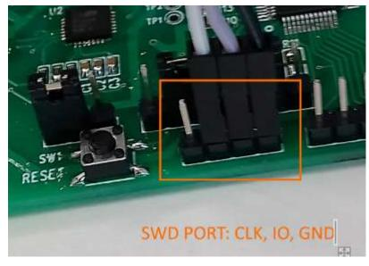
Hook up J-Link and MCU007 evaluation board as diagram shown
